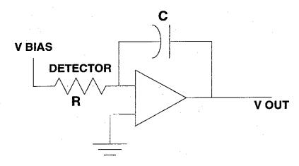
In this scenario, the current through the detector, I, is integrated such that Vout is:
